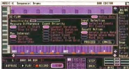
Fed up with those double-triggered notes causing problems? Get rid of them using the De-Flam option.
